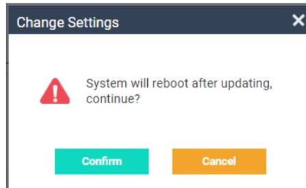
2.2.4 It may take 3 minutes to update the firmware. Please DO NOT stop the process when firmware update. During update, the LED light of front panel and screen will be off. After update process is done, unit will be reboot.
